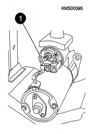
Disassembling solenoid switch
